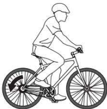
For greatest braking force, the crank arms should be horizontal when you apply the brake. The crank will rotate some before the brake starts to work, so start to apply the brake with the rear pedal slightly higher than horizontal.
